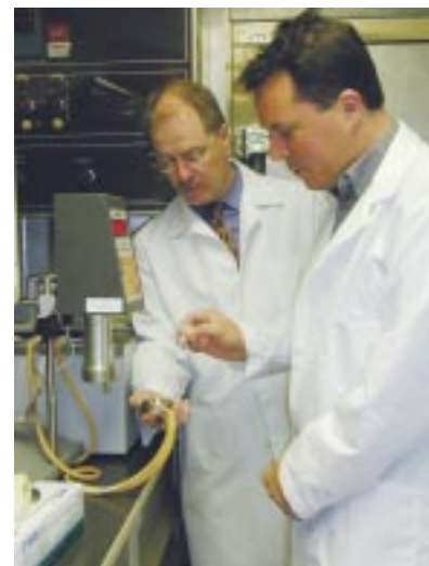
Dr. Michael Jay (left) and Dr. Russell Mumper (right) are testing the viscosity of a nanotemplate suspension used to engineer nanoparticles that are being developed by NanoMed as a potential new vaccine for AIDS.
